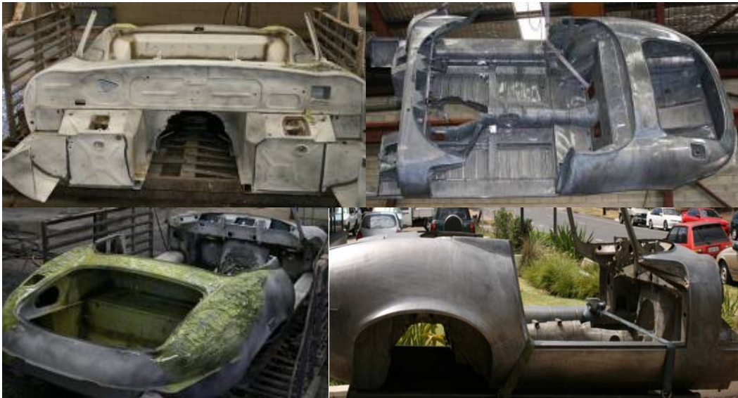
These pictures show stages in the removal of TWO/PACK URETHANE paint from Jaguar E type S3 convertible
