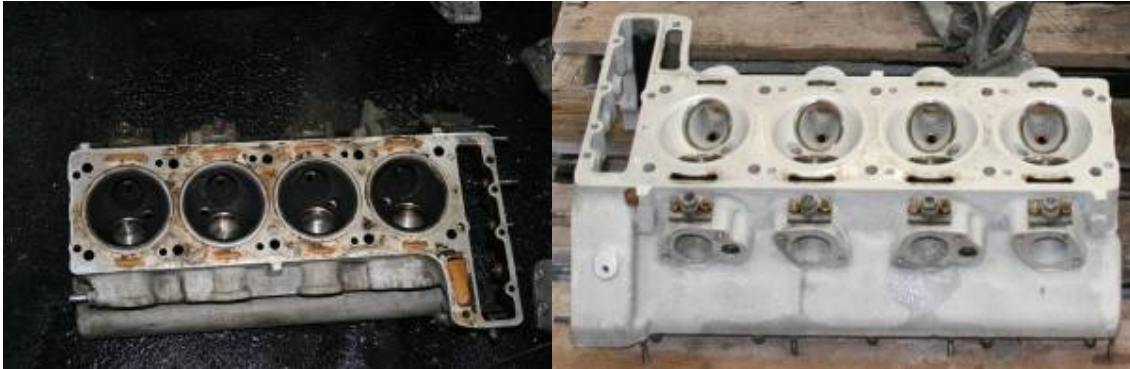
These ASTON MARTIN heads are irreplaceable and were REDI STRIPPED as part of an extensive rebuild
